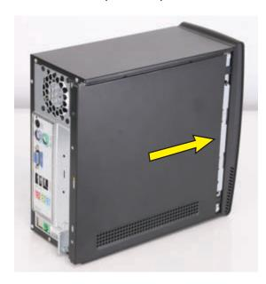
**15** Replace the screws that secure the side panel to the computer.
